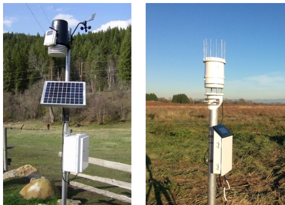
Davis Vantage Pro2/ROM Communications station (left) and the METER ATMOS41/ZL6 all-in-one station (right)
